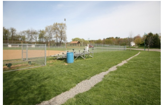
Figure 16 - ADA Seating Access a clear, firm course path needs to be provided to all fixed seating areas.
